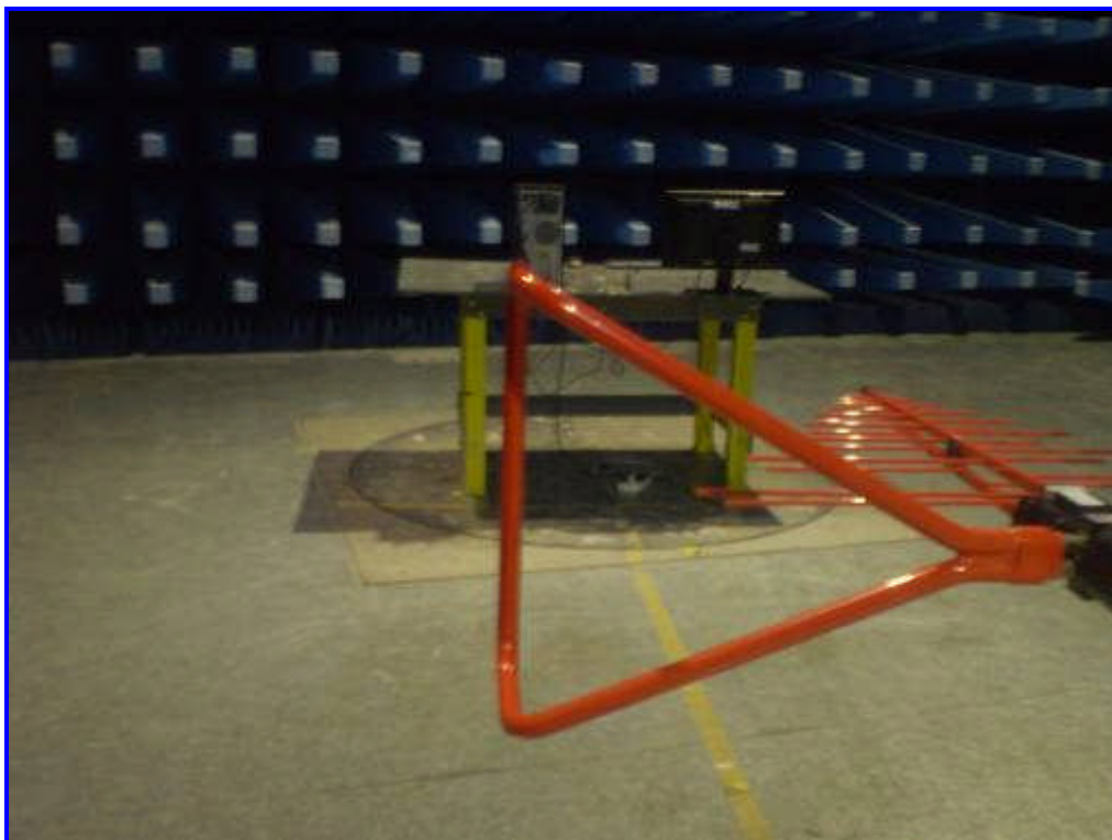
Radiated Emission Test Setup Rear View (30MHz-1GHz)
