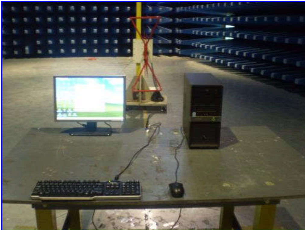
Radiated Emission Test Setup Front View (30MHz-1GHz)
