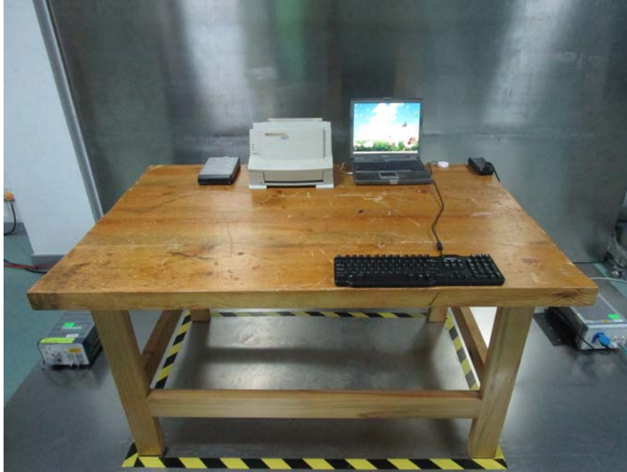
Conducted Emission - Front View
