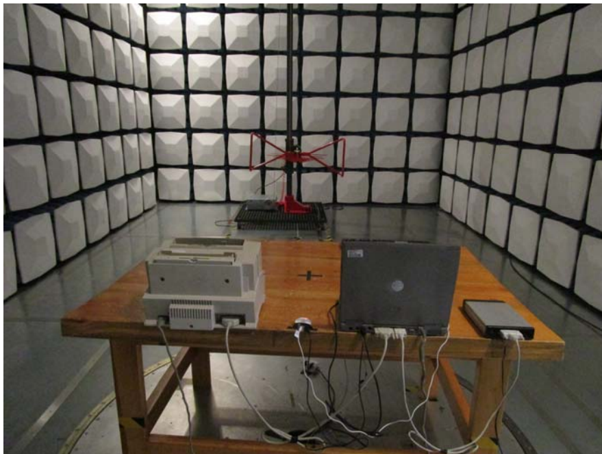
Radiated Emission - Rear View (Below 1GHz)
