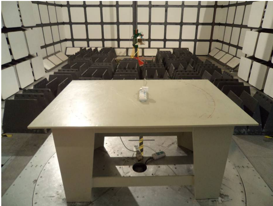
Radiated Emissions View – Above 1 GHz
