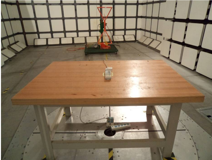
Radiated Emissions View – Below 1 GHz
