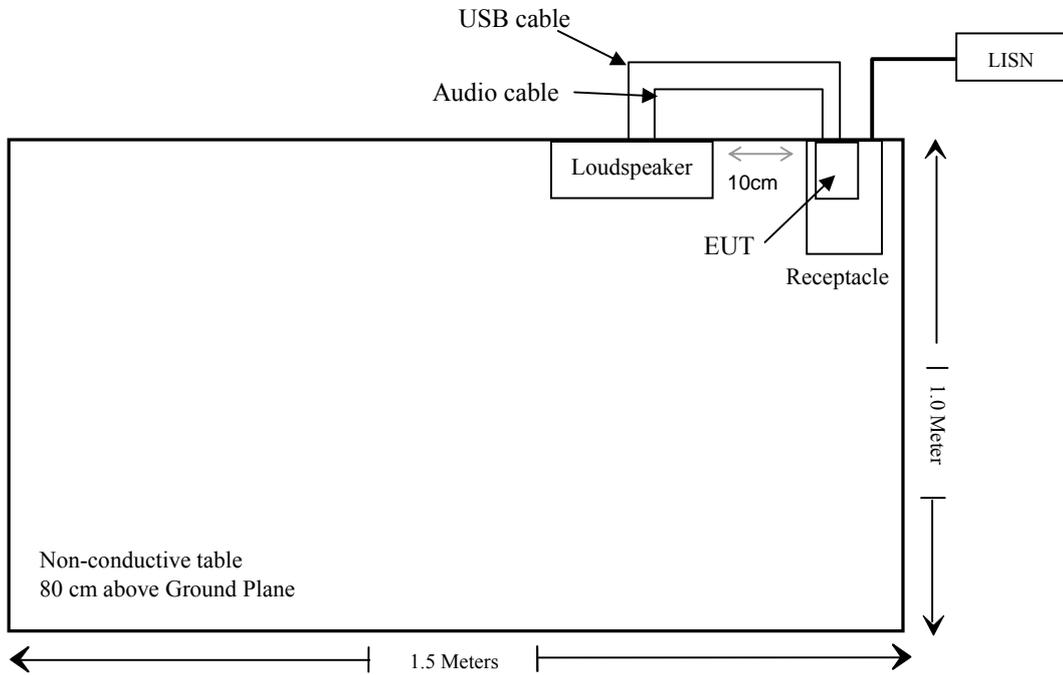
For Radiated Emission Test
