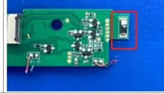
The antenna is Chip antenna. The best case gain of the antenna is 4.85 dBi.
