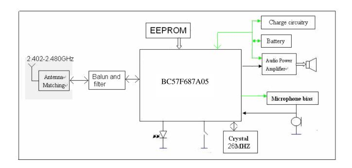
The Bluetooth Speakerphone is use CSR BC05 ROM solution, the BC05F687A05 with D.S.P. solution for Echo Cancellation & Noise Suppression.
