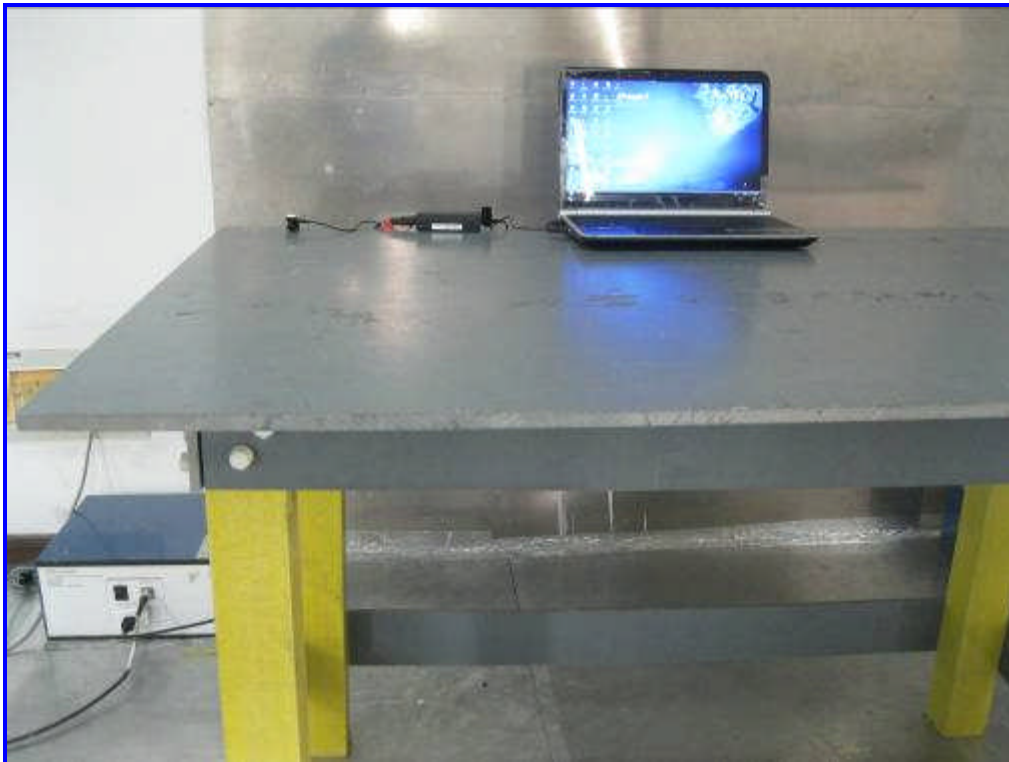
Front View of Conducted Emissions Test Setup
