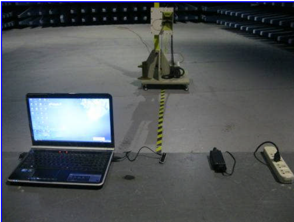
Front View of Radiated Emissions Test Setup above 1GHz
