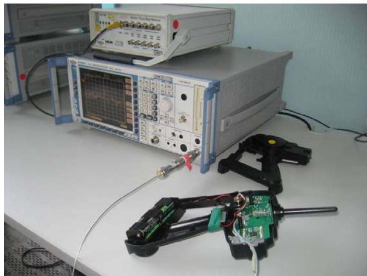
Figure 6-8: Test Configuration – Conducted Emissions
