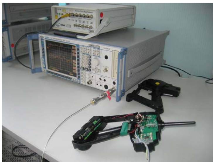
Figure 6-4: Test Configuration – 6dB Bandwidth
