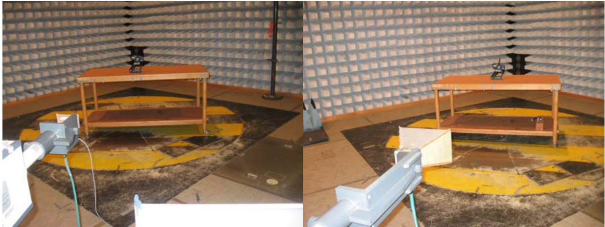
Figure 6-22: Test Configuration – Radiated Emissions (1GHz – 24.84GHz)
