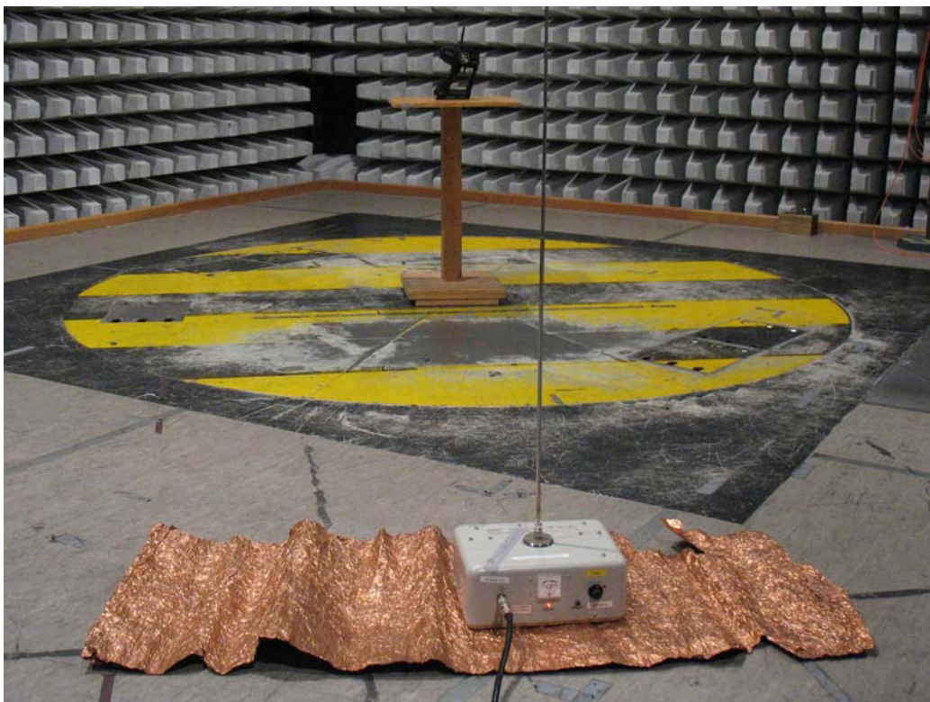
Figure 6-14: Test Configuration – Radiated Emissions (9kHz – 30MHz)
