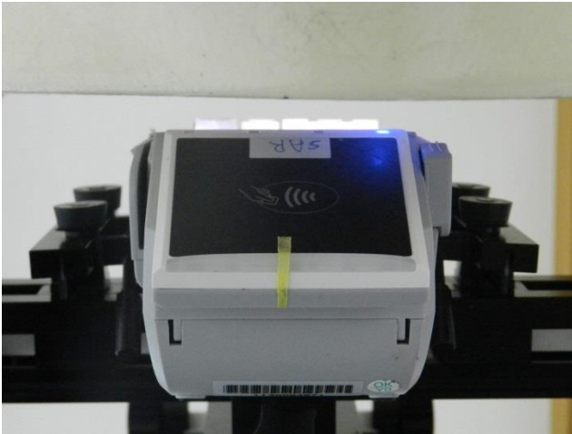
Front, Test Separation 10 mm
