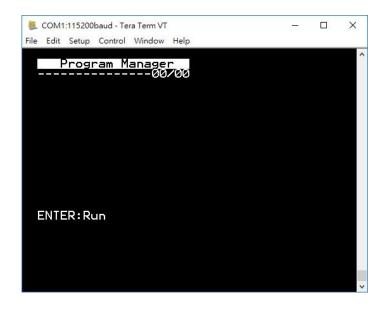
Once the power is on in normal status, UPT1000B will enter Program Manager if no default application selected. All user applications are listed in Program Manager. User can select an application and run the application, view the application info, delete the application, or set application to the default one to run once the power is on. Users may enter System Menu to configure UPT1000B settings.
