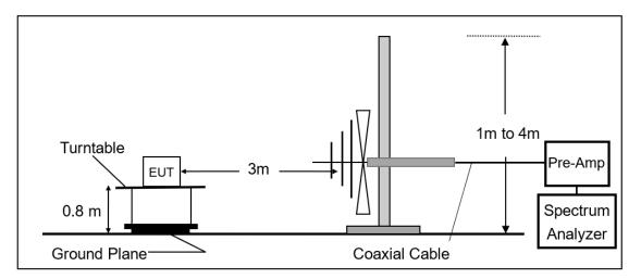
Radiated Emission Test Set-Up, Frequency Above 1GHz.
