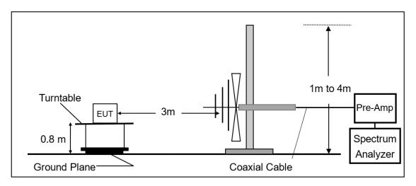
Radiated Emission Test Set-Up, Frequency Above 1GHz.
