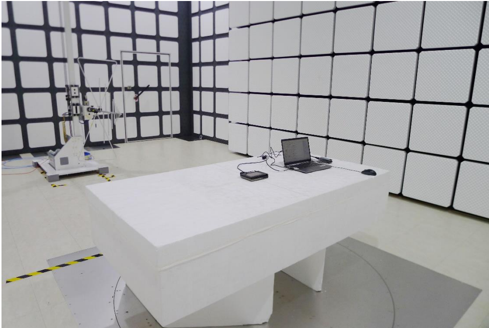
Description: Radiated Emission Test Setup for 1GHz~18GHz
