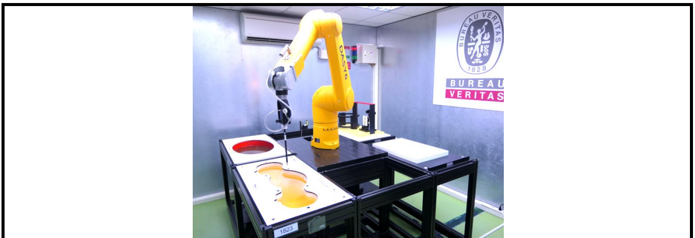
Fig-3.2 SPEAG DASY6 System
