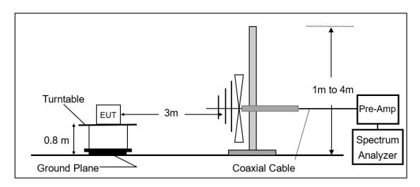
Radiated Emission Test Set-Up, Frequency Above 1GHz.
