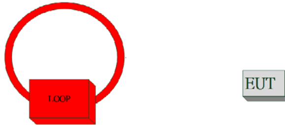
Fig. 2-2 Conduction test set up configuration
