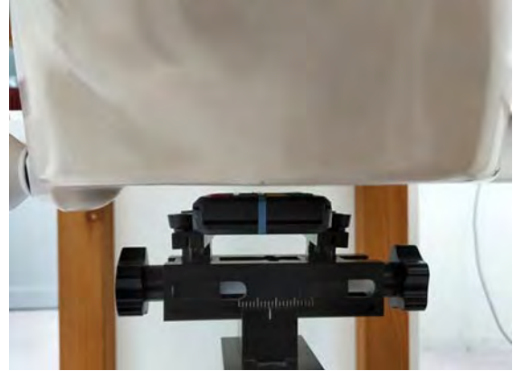
Fig.3 EUT Front side to flat phantom
