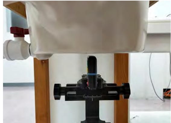
Fig.6 EUT Right side to flat phantom
