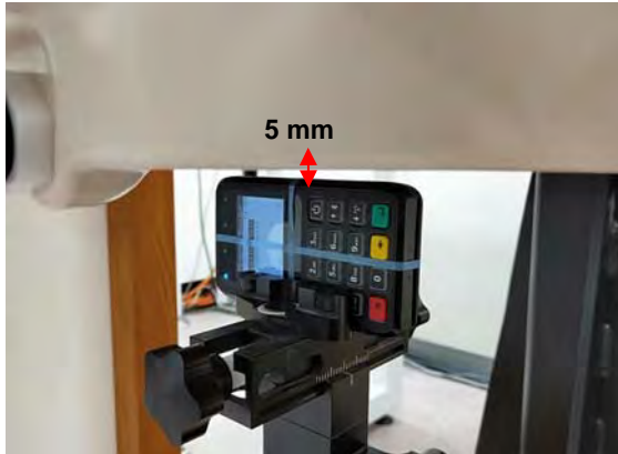
Fig.6 EUT Right side to flat phantom
