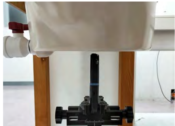
Fig.5 EUT Top side to flat phantom
