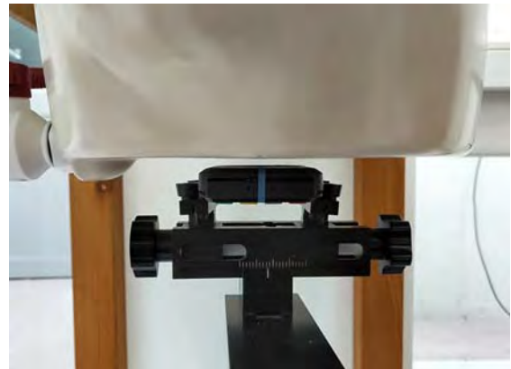
Fig.4 EUT Back side to flat phantom
