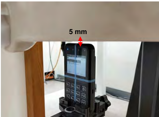
Fig.5 EUT Top side to flat phantom
