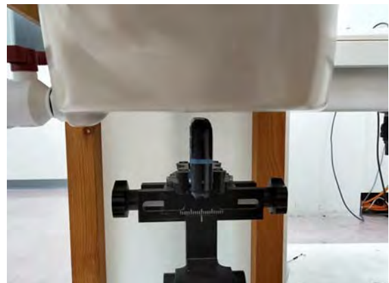
Fig.7 EUT Left side to flat phantom
