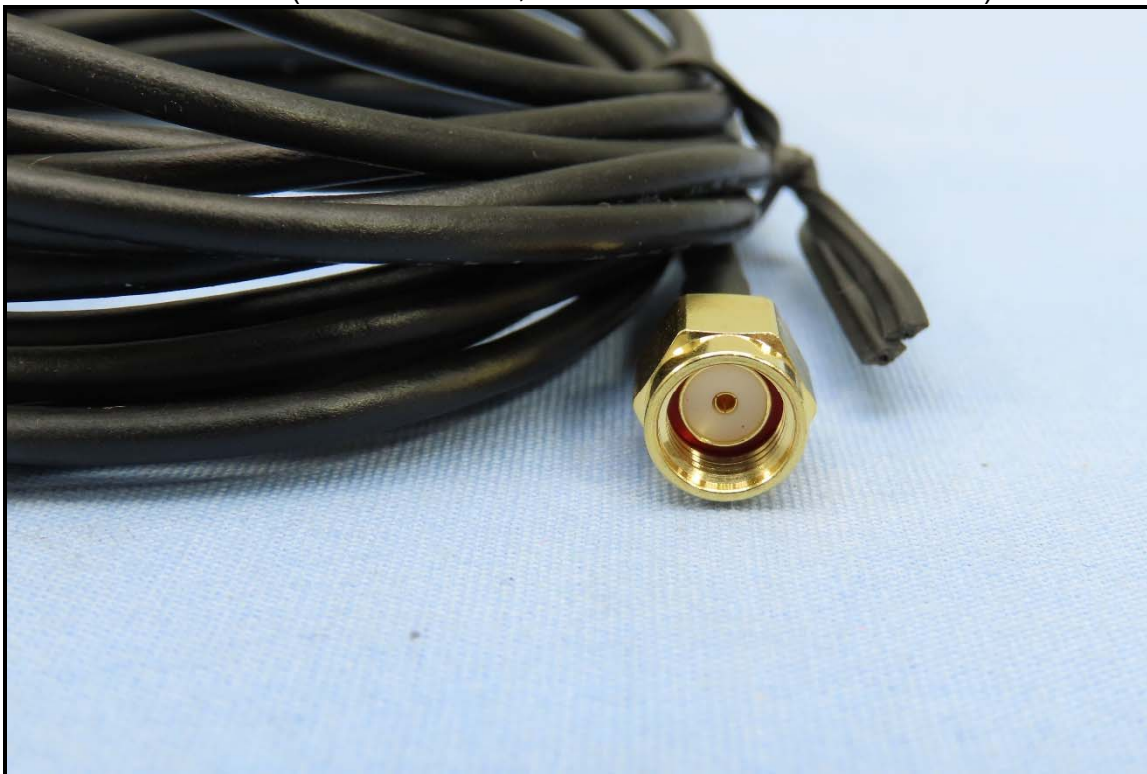
Antenna (Brand: Aristotle, model: RFA-25-T100-41-3M-A2)
