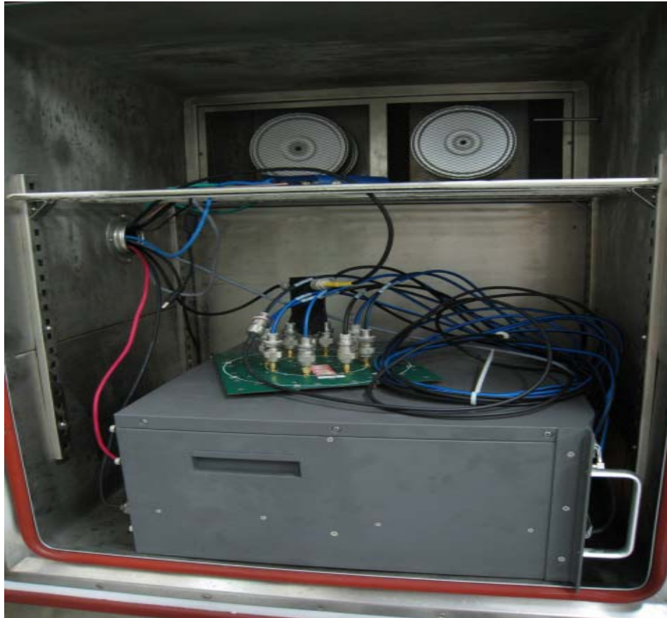
Photograph of Frequency Stability Test Setup
