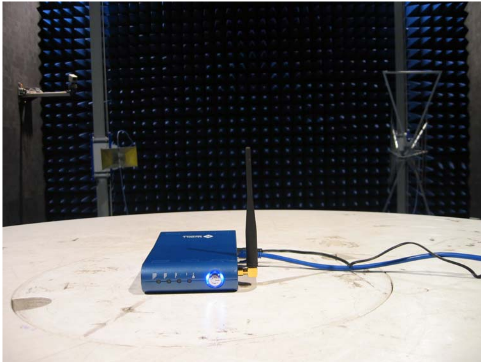
Photograph of Radiated Spurious Emissions Test Setup
