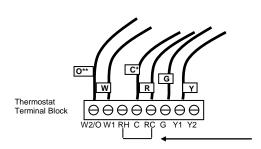
Connect the wires as marked from the HVAC system to the corresponding terminals on the thermostat back.
