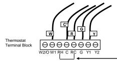
Connect the wires as marked from the HVAC system to the corresponding terminals on the thermostat back.
