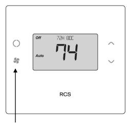
Press the FAN button to change the Fan mode
