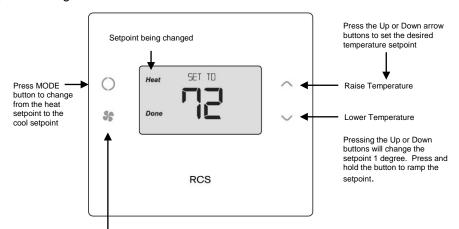
Press "Done" (FAN button) to set the setpoint and exit back to the main thermostat screen or wait for the screen to automatically time out.
