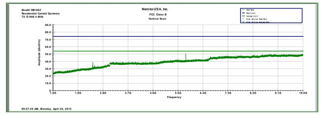
CFR 47, PART 15, Paragraph 15.249 and Industry Canada RSS-210, Issue 8 Operation within the bands 902-928 MHz, 2400-2483.5 MHz, 5725-5875 MHz, and 24.0-24.25 GHz.
