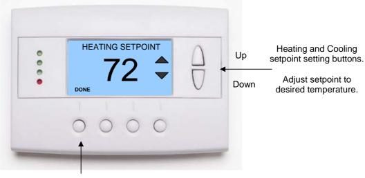
Press **Done** button to select new setpoint and exit back to main thermostat screen.
