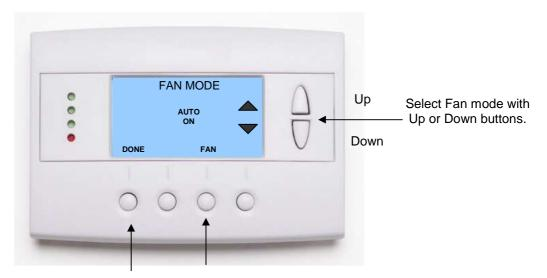
Press **DONE** button to select mode and exit back to main Thermostat Control Screen.
