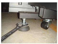
Next rotate the lower nut counterclockwise until the foot reaches the floor and the wheels do not.
