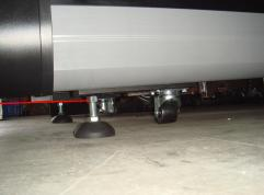
After the four feet reach the floor, confirm the device is balanced and screw the upper nuts.
