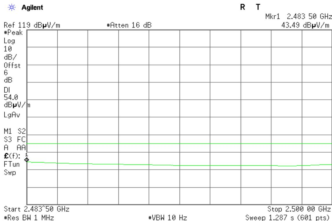
**Test Plot****Conducted Band Edges (IEEE 802.11b mode / CH Low)**
