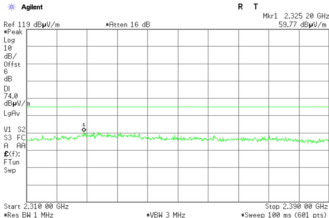
**Detector mode: Average****Polarity: Horizontal**
