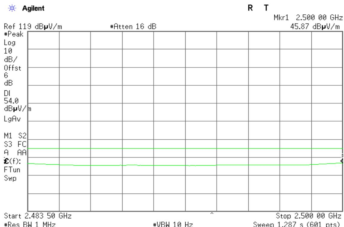
**Detector mode: Peak****Polarity: Horizontal**
