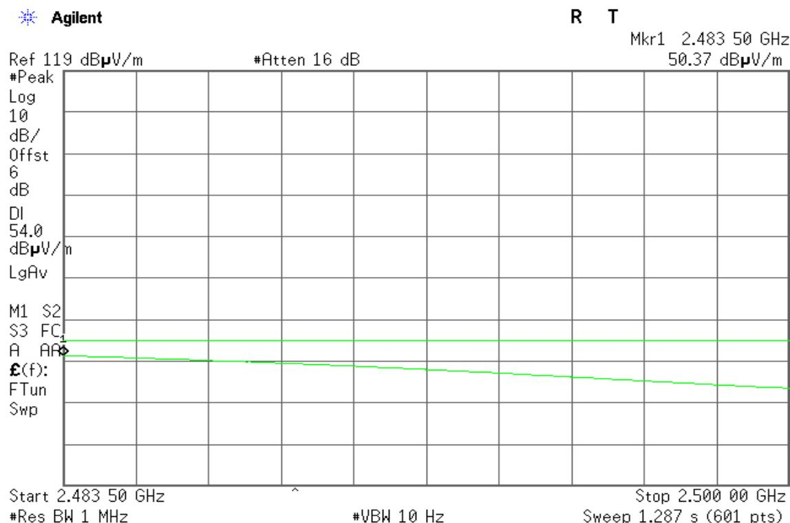
**Detector mode: Peak****Polarity: Horizontal**
