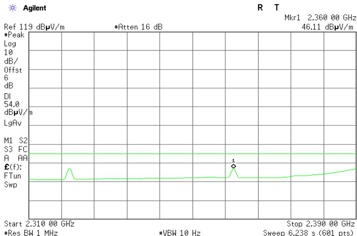
**Detector mode: Peak****Polarity: Horizontal**
