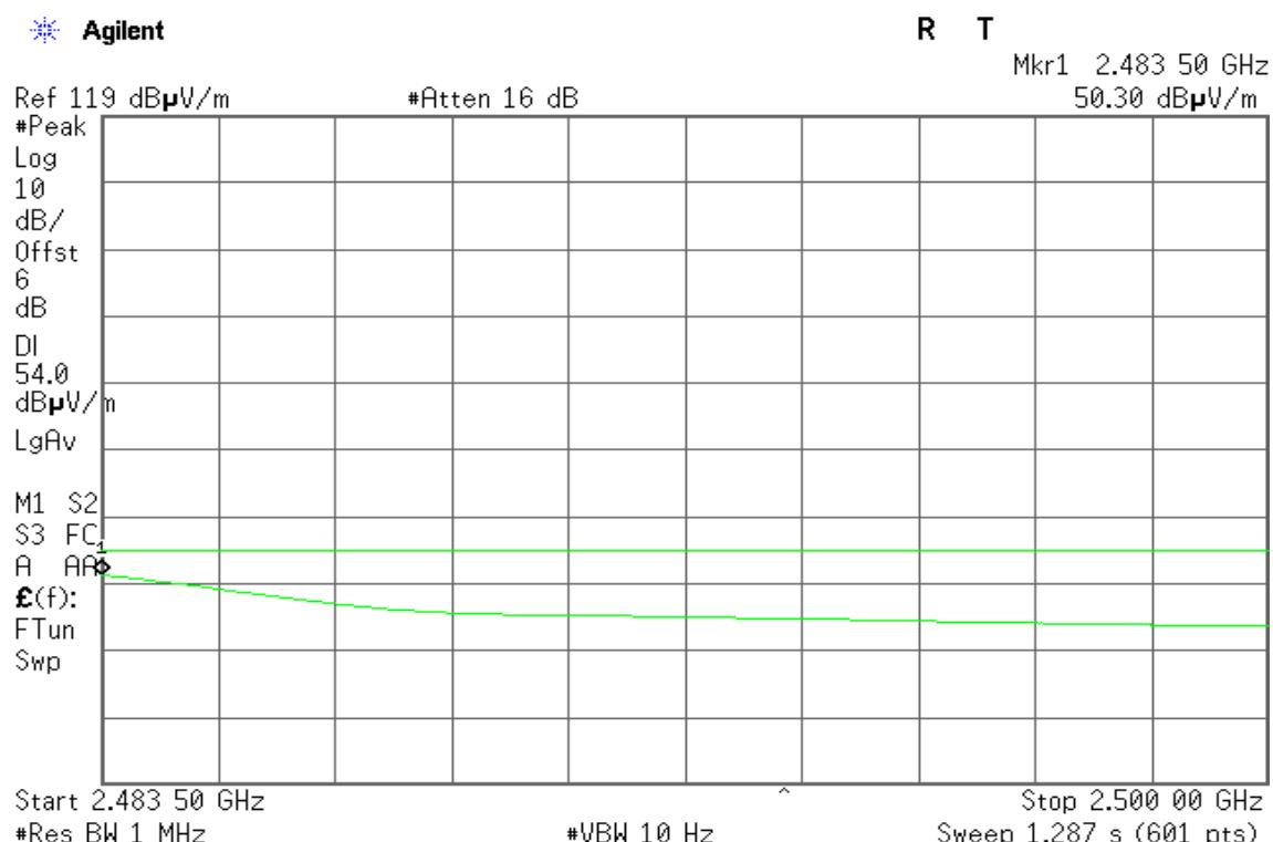
**Detector mode: Peak****Polarity: Horizontal**
