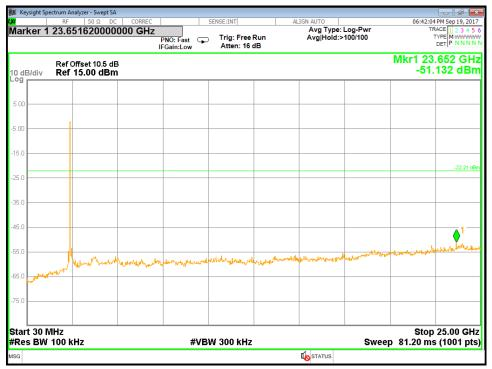
Test mode : 802.11n\_HT20 / Lowest Frequency\_Conducted Spurious Emission
