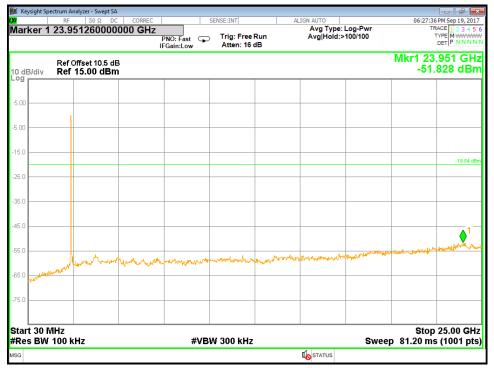
Test mode : 802.11b / Lowest Frequency Conducted Spurious Emission
