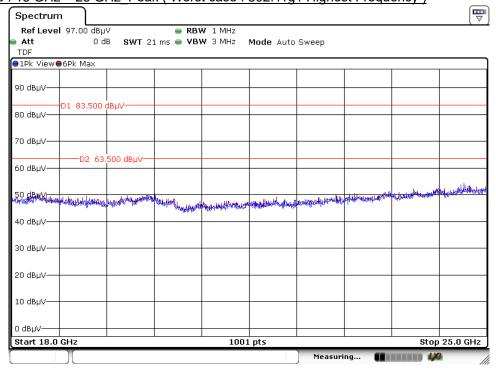
Test mode : 18 GHz ~ 25 GHz Peak ( Worst case : 802.11g / Highest Frequency )
