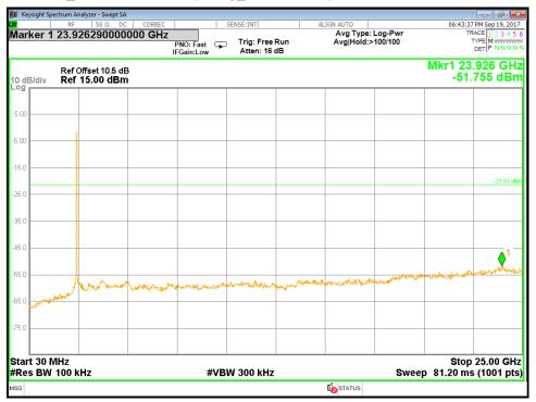
Test mode : 802.11n HT20 / Middle Frequency Conducted Spurious Emission
