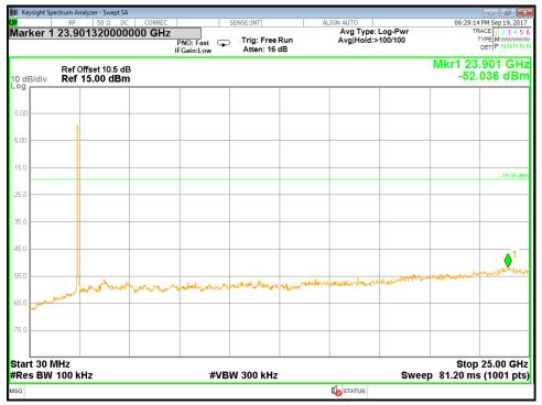
Test mode : 802.11b / Middle Frequency\_Conducted Spurious Emission
