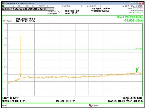
Test mode : 802.11g / Middle Frequency\_Conducted Spurious Emission
