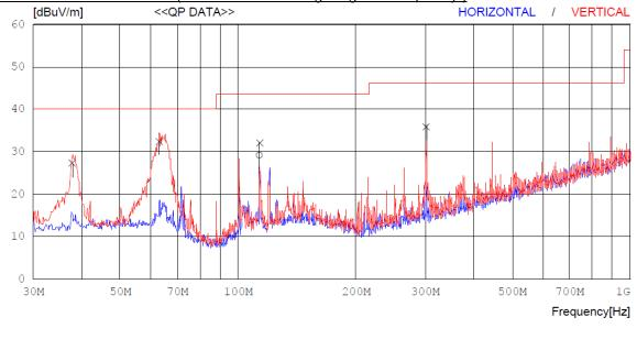
Test mode : 30 MHz ~ 1 GHz ( Worst case : 802.11g / Highest Frequency )
