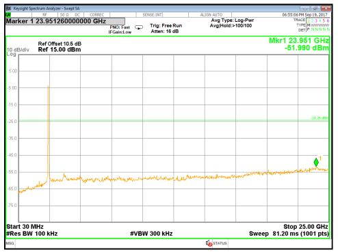
Test mode : 802.11n HT40 / Middle Frequency Conducted Spurious Emission
