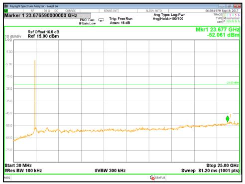
Test mode : 802.11g / Lowest Frequency Conducted Spurious Emission
