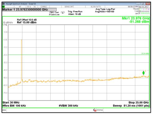
Test mode : 802.11n HT40 / Lowest Frequency Conducted Spurious Emission
