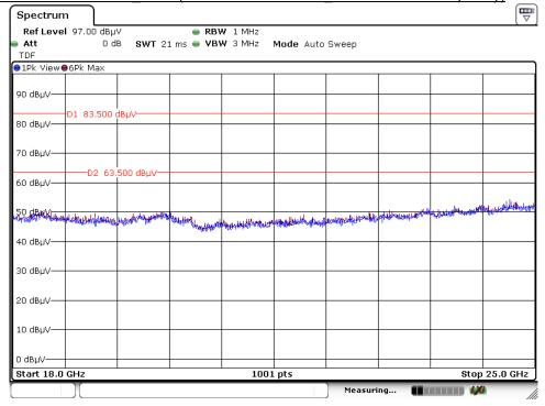
Test mode : 18 GHz ~ 25 GHz Peak (Worst case : 802.11n HT20 / Lowest Frequency)
