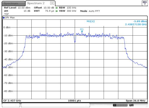
Test mode : 802.11n HT20 / Middle Frequency Conducted Spurious Emission
