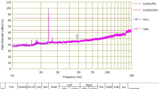
Test mode : 1 GHz ~ 18 GHz (Worst case : 802.11n HT20 / Lowest Frequency)
