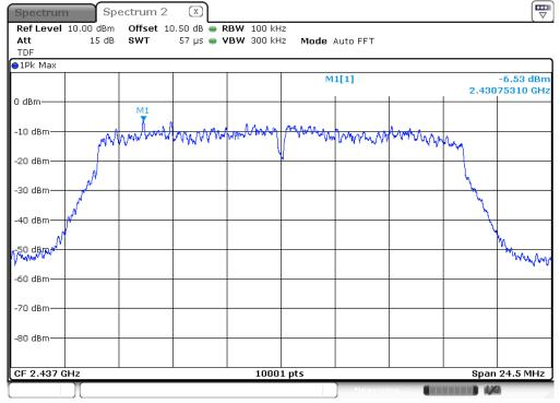
Test mode : 802.11g / Middle Frequency\_Conducted Spurious Emission
