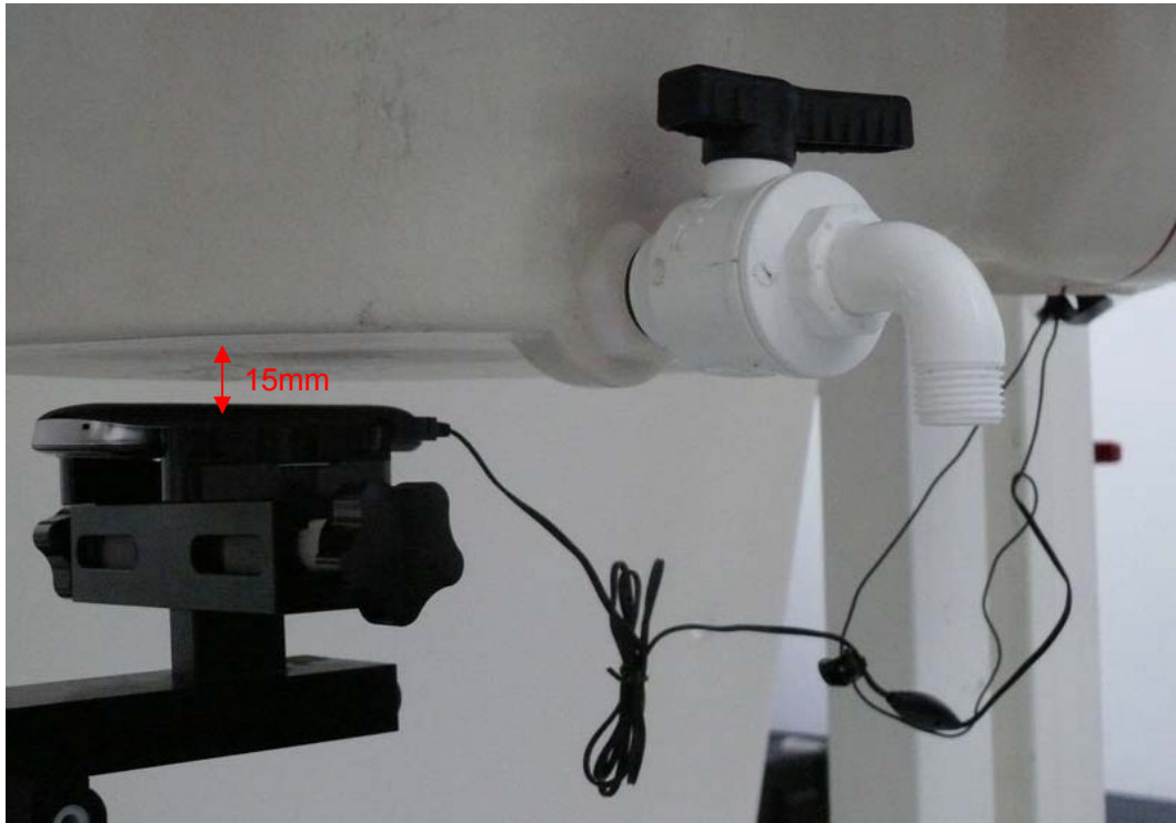
Picture 13: Body with earphone, The EUT display towards ground, the distance from handset to the bottom of the Phantom is 15mm
