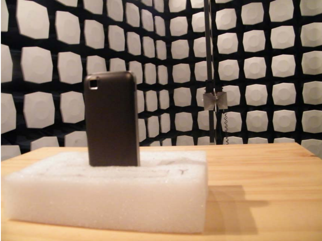
Picture 2: Radiated Spurious Emissions Test setup
