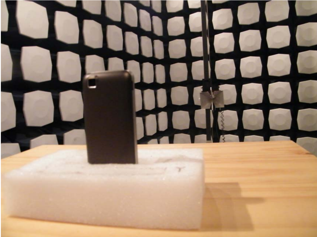
Picture 2: Radiated Spurious Emissions Test setup
