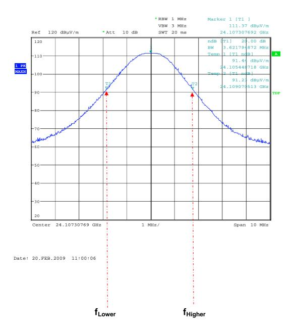
$\begin{array}{lll} f_{Lower} & = & 24.105448718 \ \text{GHz} \\ f_{Higher} & = & 24.109070513 \ \text{GHz} \\ \text{Occupied Bandwidth} & = & 3.62179 \ \text{MHz} \\ \end{array}$
