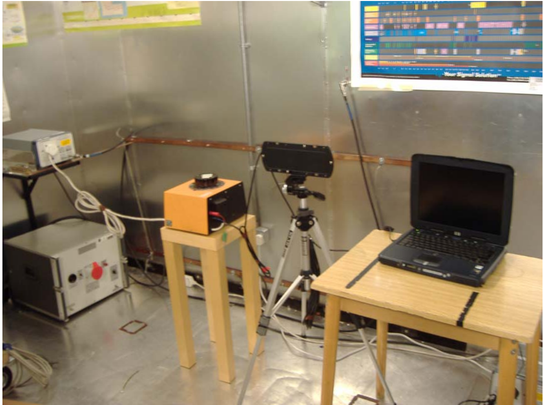
AC Powerline Conducted Emissions Test Setup
