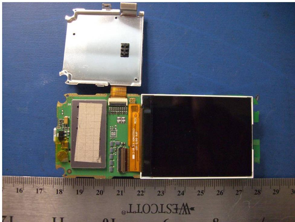
**RF Board with Shield off**
