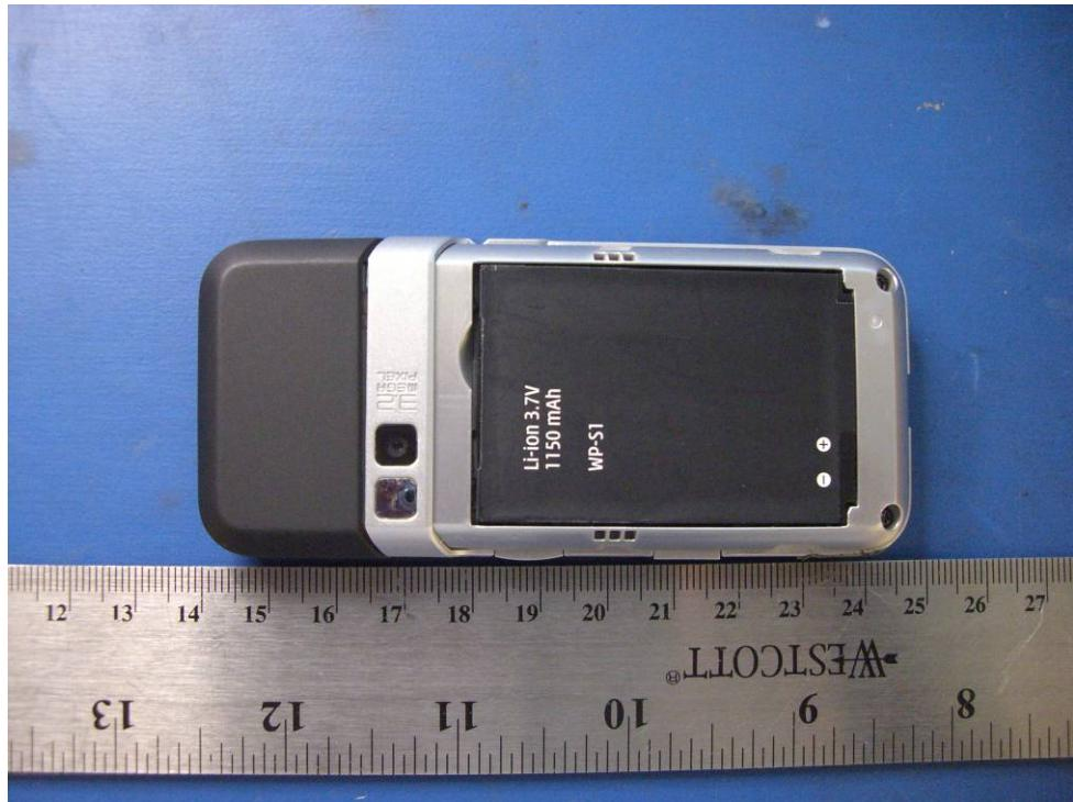
**EUT Back Side with Cover off**
