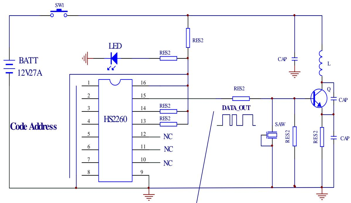
The encoded waveform is serially outputted
