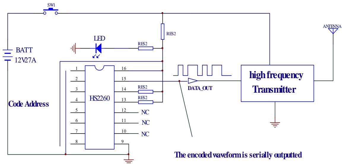
HS2260A is a general-purpose remote coding integrated circuit
