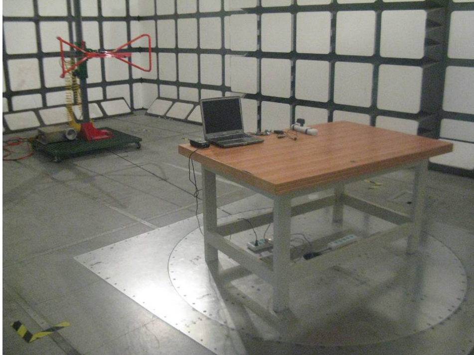
Below 1 GHz: Radiated Emissions - Rear View (Transmitting)
