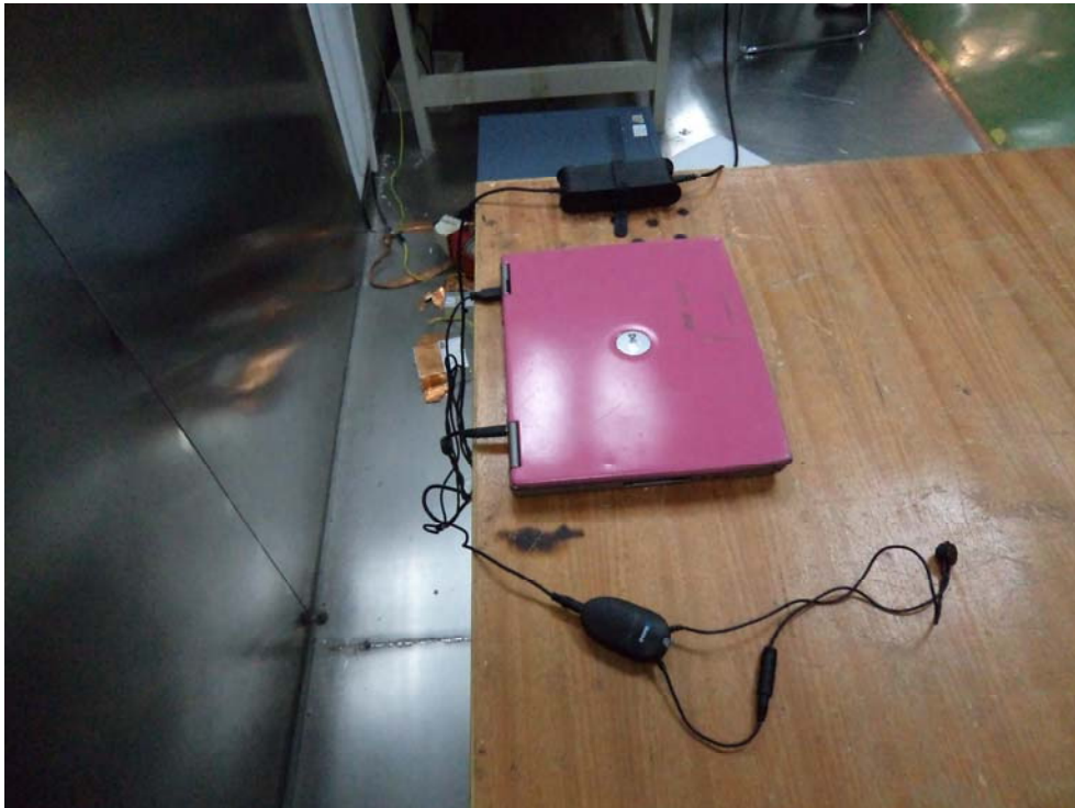
Conducted Emissions - Side View (PC Charging)
