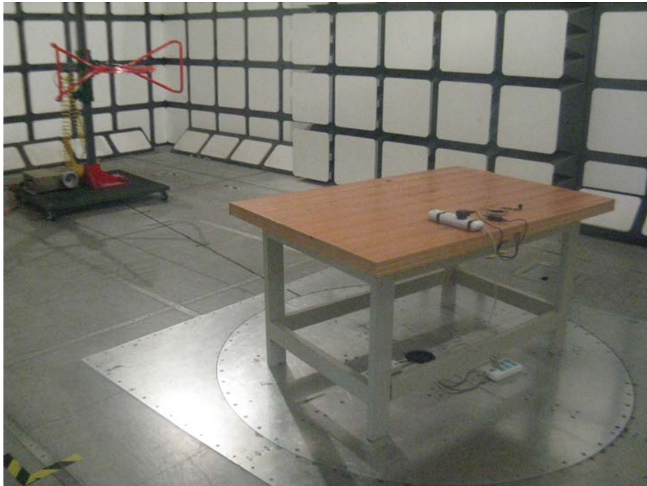
Below 1 GHz: Radiated Emissions - Rear View (Adapter Charging)
