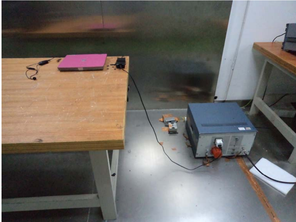
Conducted Emissions - Side View (PC Charging)
