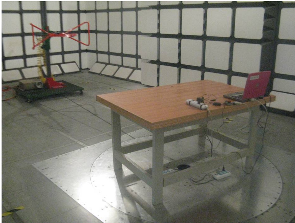
Below 1 GHz: Radiated Emissions - Rear View (Transmitting)
