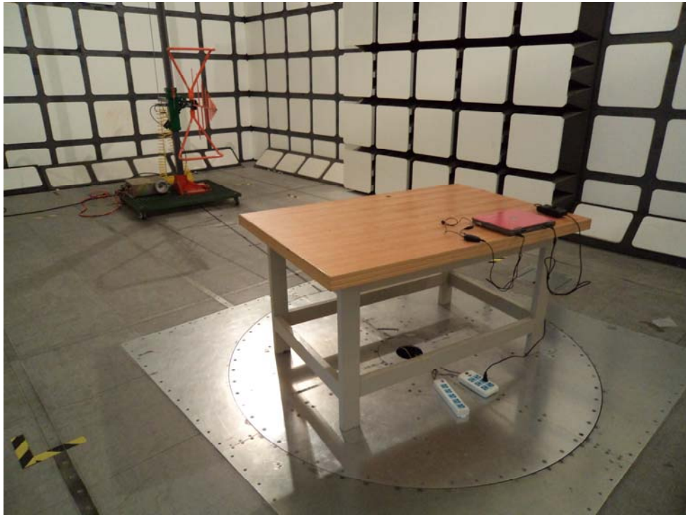
Below 1 GHz: Radiated Emissions - Rear View (PC Charging)
