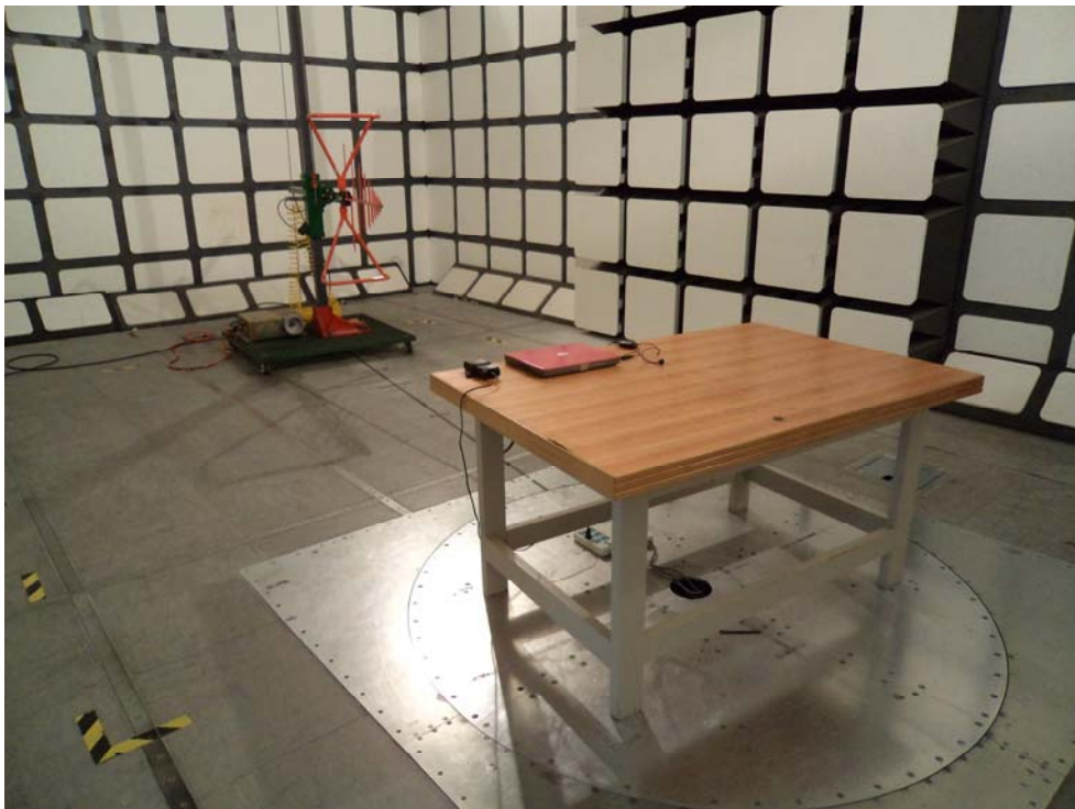
Below 1 GHz: Radiated Emissions - Rear View (PC Charging)
