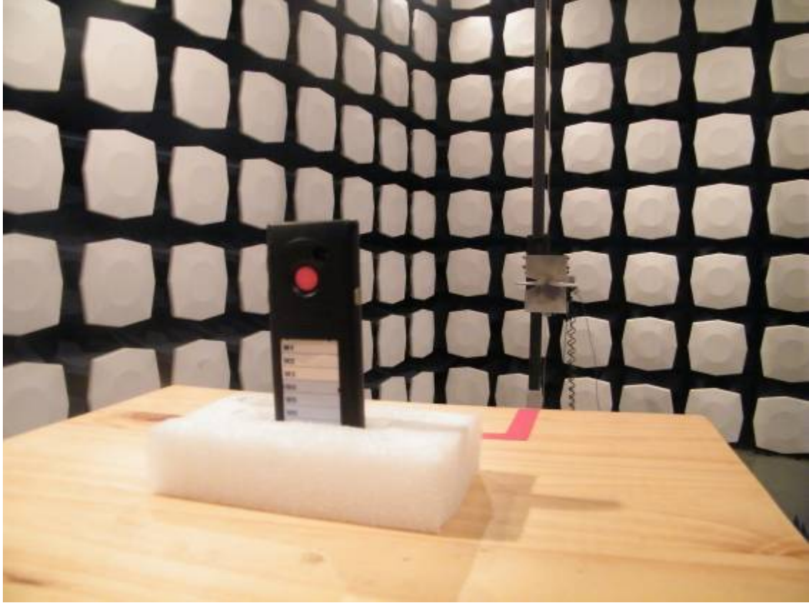
Picture 2: Radiated Spurious Emissions Test setup
