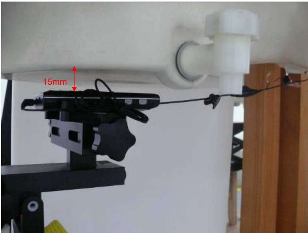
Picture 14: Body with Earphone, The EUT display towards phantom, the distance from handset to the bottom of the Phantom is 15mm
