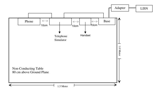
Radiated Emission test for handset
