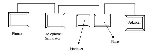
Radiated Emission test for handset
