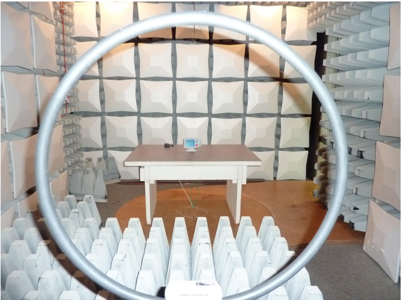
181775_fcc_01: Test setup fully anechoic chamber > 30 MHz
