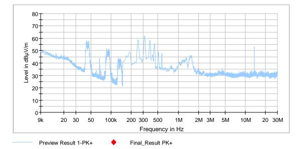
172189magFCC 1356.Rtf: Emissions from 9 kHz to 30 MHz reading a 13.56 MHz TAG
