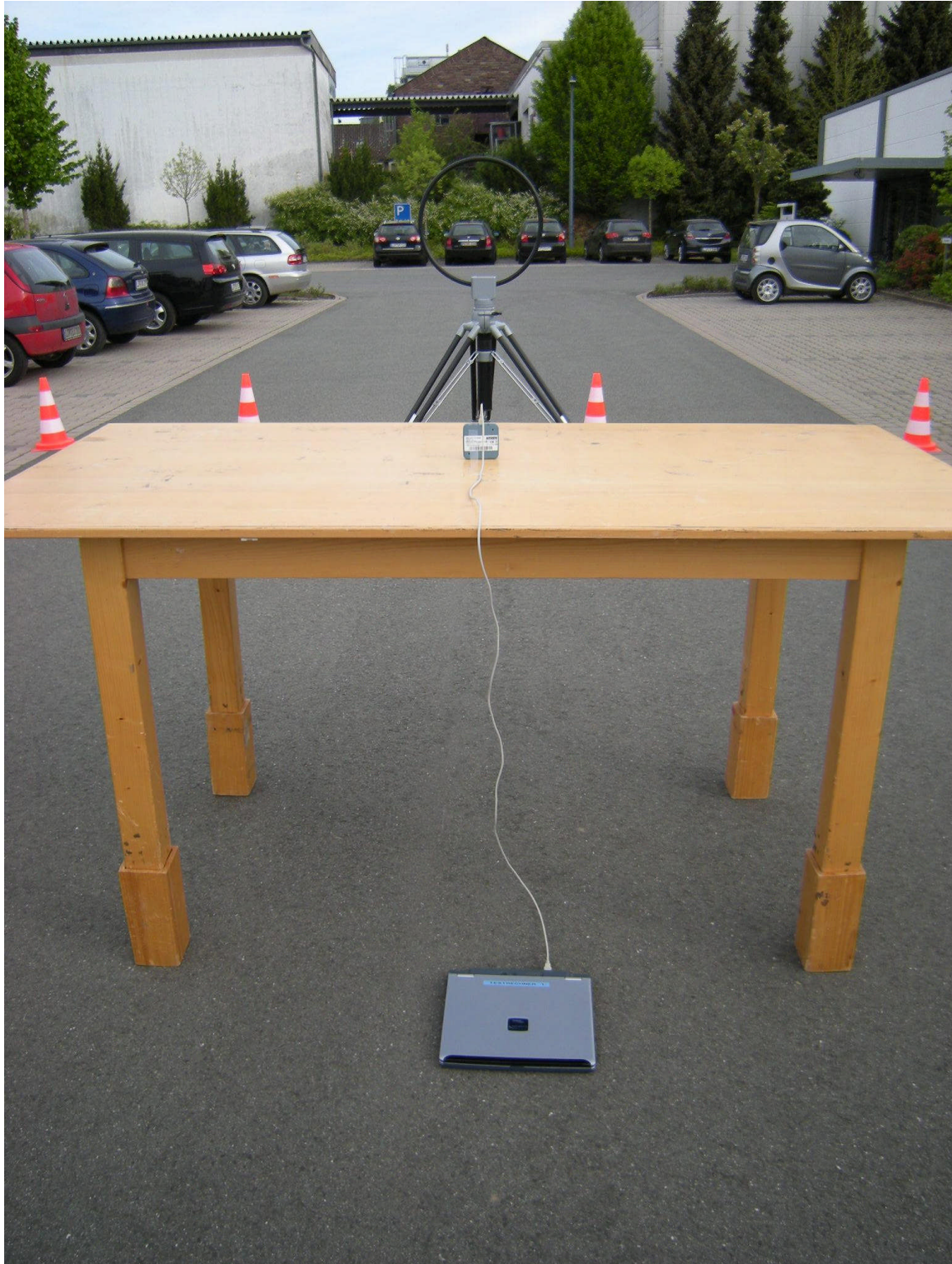
91052emi_fcc9.jpg Test set-up outdoor test site
