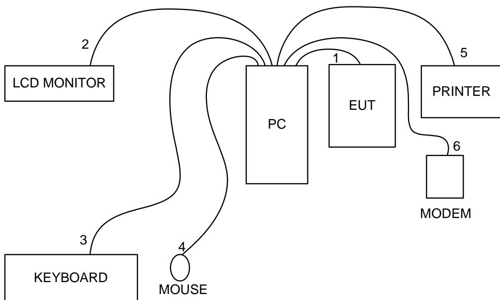
1. The USB cable is connected from the EUT to the support unit 1.
