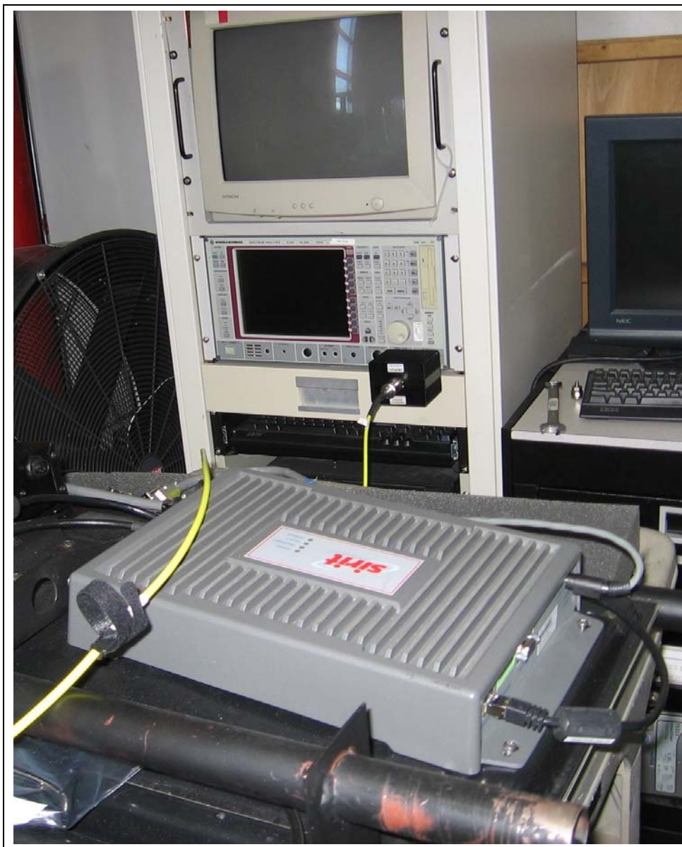
Figure 16 Test setup for SPURIOUS EMISSIONS – Antenna conducted
