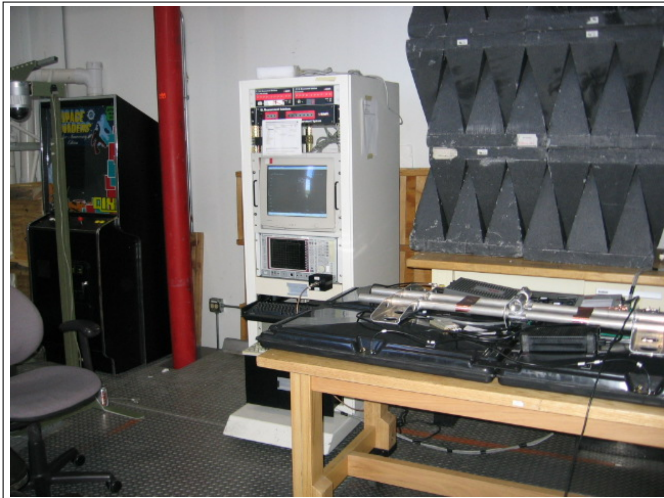
Figure 6 Test Setup for 20dB Bandwidth
