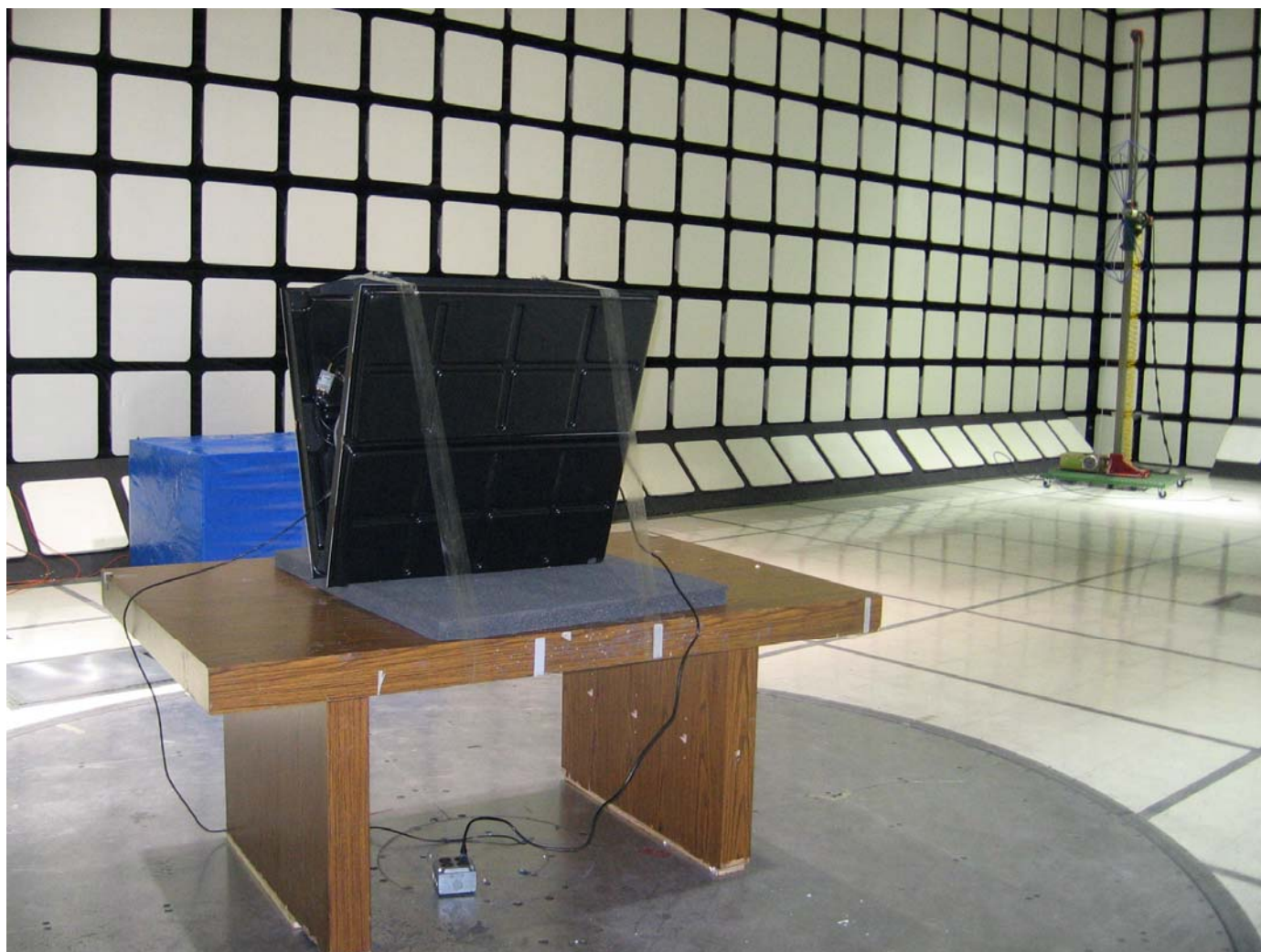
Figure 22 Test setup for SPURIOUS EMISSIONS
