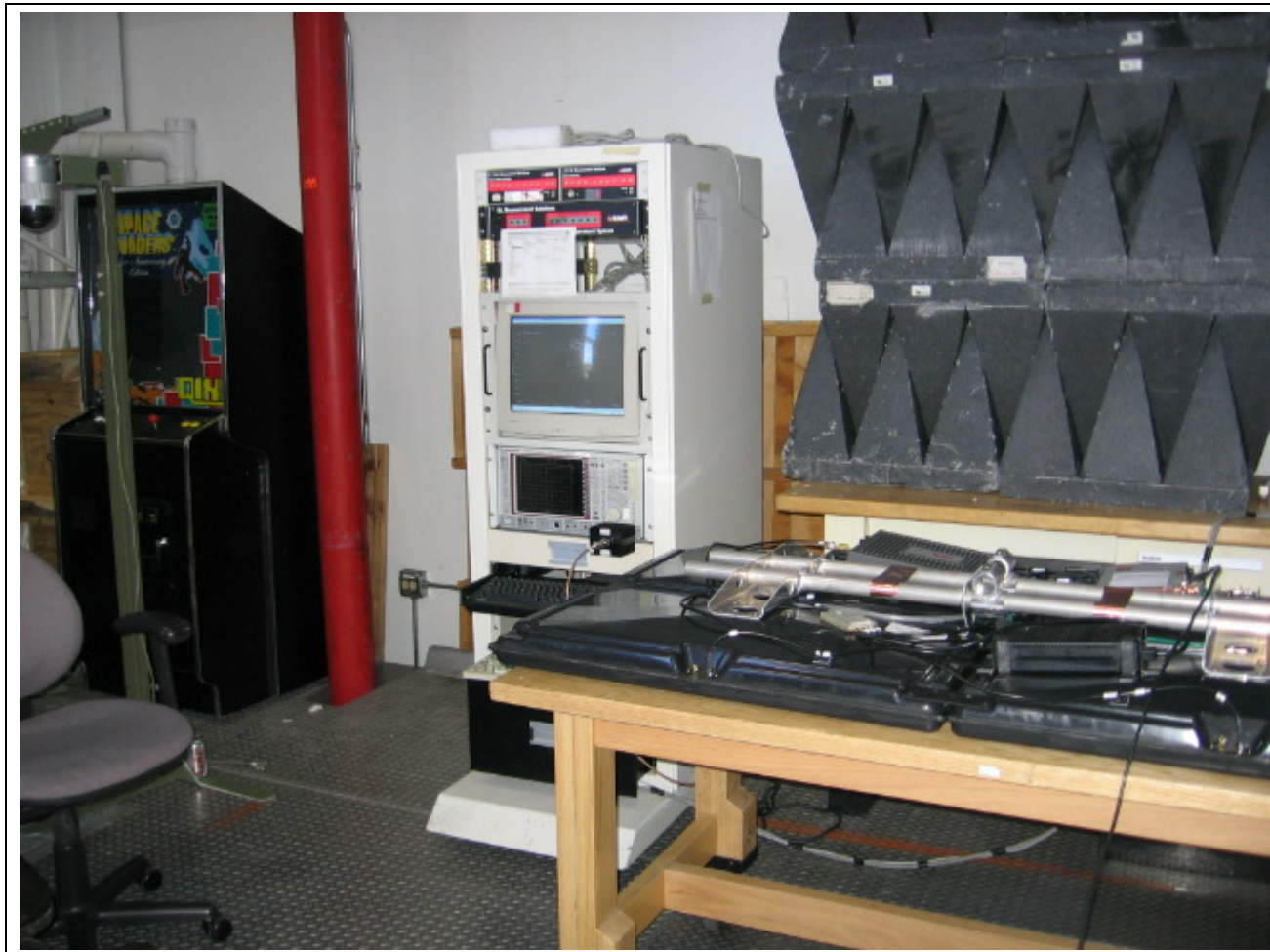
Figure 8 Test Setup for Number of Hopping Frequencies
