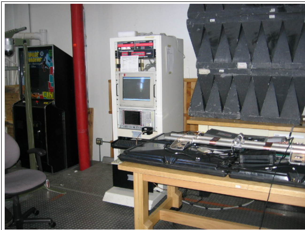
Figure 14 Test setup for Band Edge Compliance – Conducted
