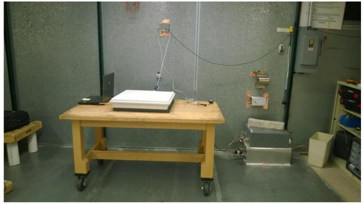
\*Setup shown in the photo is for the EU Telecomuunication Port Conducted Emissions testing. For FCC the ISN was no in the circuit and the blue Ethernet line with the ferrite on was connected directly to the PoE adapter on the table.
