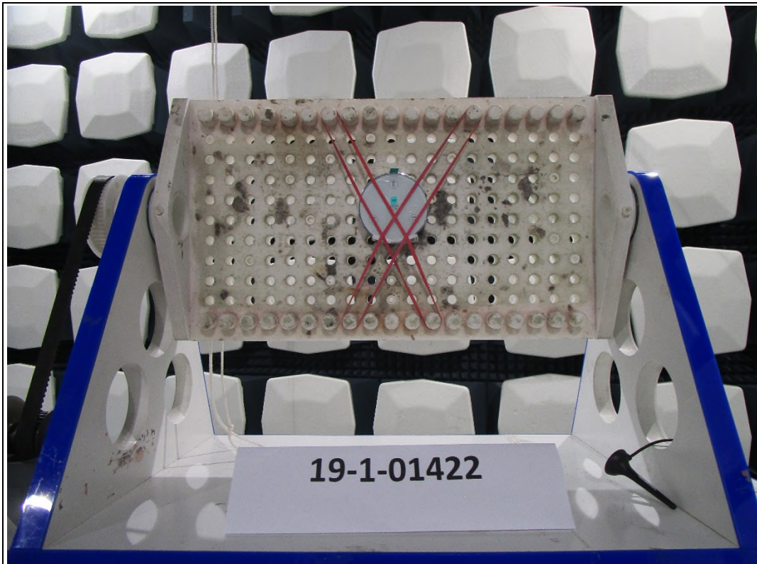
Photograph 3: Radiated measurements test set-up, 1 GHz – 26 GHz
