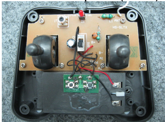
Inner Circuit Top View
