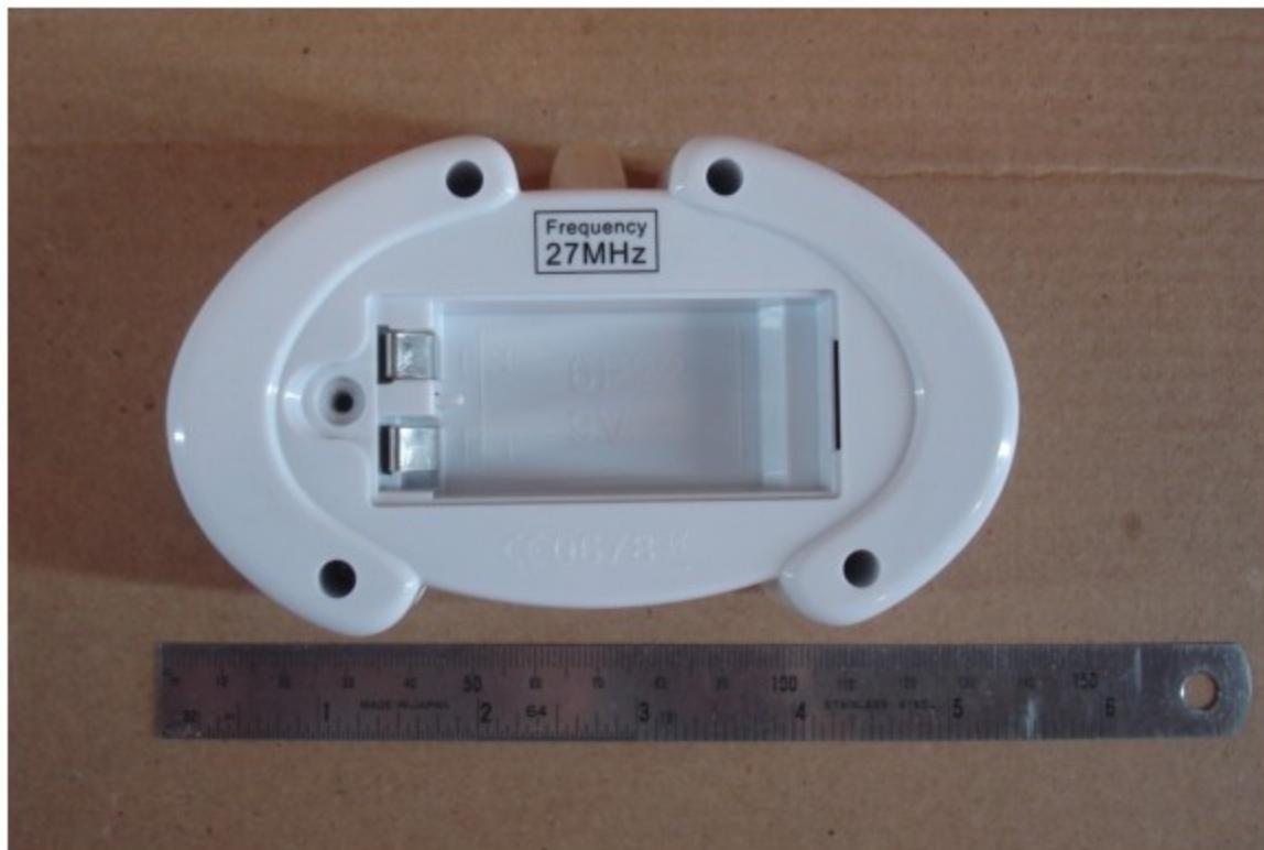
Because the majority of the device housing is too small, there is extremely limited space available to attach the required label carrying both the FCC identifier and statement. For this reason, **Playmind Ltd.** proposes placing FCC statement in the user manual.
