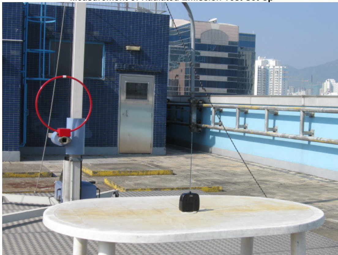
Measurement of Radiated Emission Test Set Up
