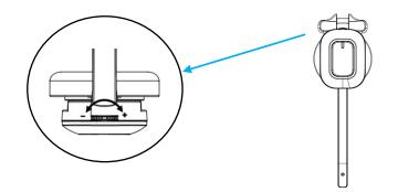
To change the speaker volume: tilt the volume switch towards the 'plus' sign to increase the volume and tilt the switch towards the 'minus' sign to decrease the volume and press the switch to activate the microphone mute mode.
